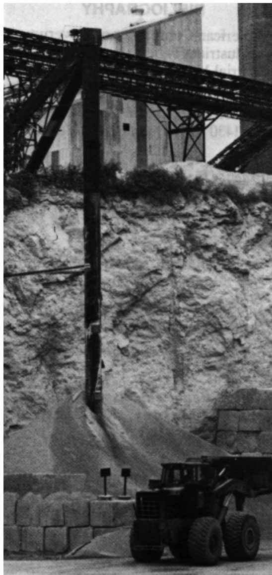
Figure 9. To minimize free fall and dusting, drop tubes contain falling material from belt and allow it to trickle out from ports opening just above the storage pile.
