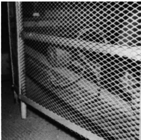
Figure 2. Enclosing the sides of the belt will prevent contact with nip points. Grease fillings are placed so guard does not have to be removed while servicing.
